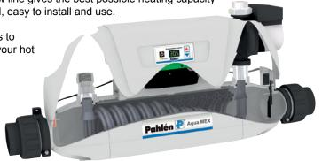
Aqua MEX fully equipped has a three-step single-phase built-in circulation pump for the primary (hot) water as well as built-in temperature sensor, flow switch and check valve. It is also equipped with two drain plugs on the secondary circuit (pool water) for easy drainage of the heat exchanger.
